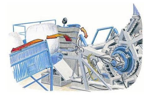
5. The wrapped bale is now fed on to the bale conveyor. The whole process lasts 2 - 3 minutes and is fully computerised.
