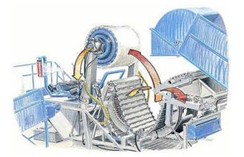
3. The bale chamber opens up and the bale is transferred to the wrapper unit.
