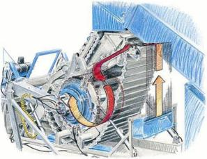
2. To keep the shape of the bale, a net or a film is fed into the chamber
