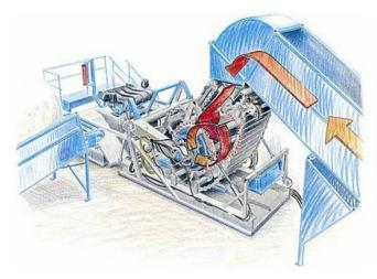
1. The material is fed into the bale chamber until full pressure is reached.
